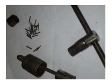
The bearing was in terrible state, corroded with rust, one needle missing and the collar like a ploughed field. Phil Atkinson, a multiple championship winner, came to grief at Donington a week before my incident, owing to suspension failure, so hopefully I will be spared that.
