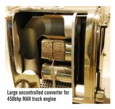
Any unburnt fuel, such as may be admitted to the converter when unsuccessfully attempting to start the engine, can – after starting – raise converter temperature to a level where the honeycomb will melt, partially blocking the exhaust, and promoting other damage such as burnt exhaust valves. Such unused fuel is reduced in many modern engines by a camshaft position sensor,
