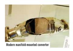
The probe output, of course, is a feedback signal, and in monitoring the exhaust output it is used to modify the injection period, and also in many cases the ignition timing, to control the basic exhaust quality. This basic exhaust - probe signal - injection control - modified exhaust cycle is referred to a closed control loop, and therefore this type of converter is known as a 'Closed Loop' device, as is fitted to virtually all modern cars and many motorcycles.
