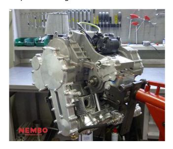
The 2-litre engine provides most of the chassis, and puts the mass where it's wanted. It's said to be more compact than most current 1,000cc three- or four-cylinder traditional engines, thus allowing a very long (carbon fibre) swingarm, that provides "excellent stability and great traction. Another record." BTW, it's called the 32 because it's a 3-cylinder, 2-litre.
