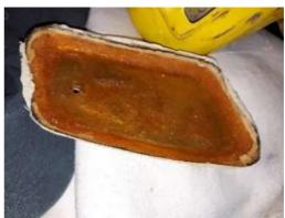
First made a pattern from cardboard then I shaped the aluminium as a former upon which to build a fibreglass lid. Once the shape was properly created, the aluminium
