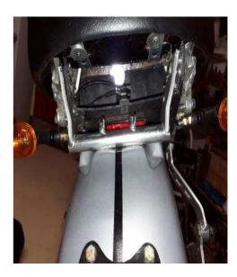
Note the wing nuts and spring washers as the whole mudguard needs to come off when removing the rear wheel. Another piece of robbery came when came the technicality of how to secure the seat base on to the sub frame.
